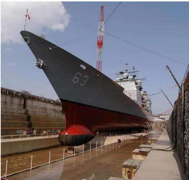
The Ticonderoga-class guided missile cruiser USS Cowpens on dry dock in Japan. See the AN/SQS-53B/C/D sonar mounted at the bow, USN
