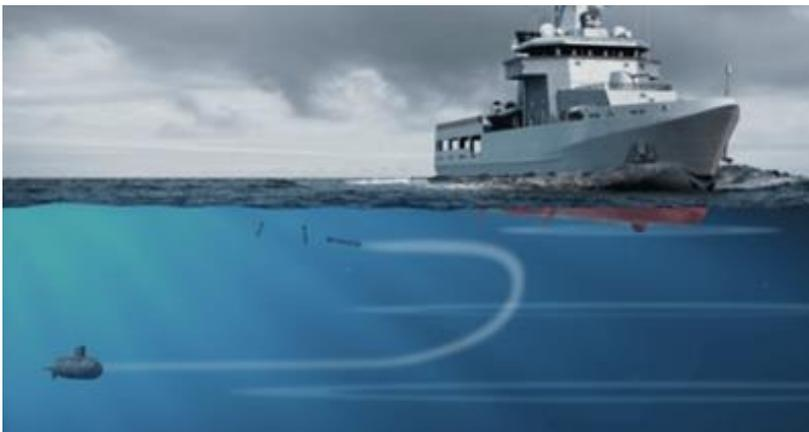
Israeli underwater defence systems supplier DSIT Solutions will present a complete torpedo defence system for surface ships at the Euronaval 2022 exhibition in Paris from 18-21 October 2022. The product presented by DSIT includes the Hull Mounted Sonar (HMS) system integrated with RAFAEL's anti-torpedo defence system (ATDS).
